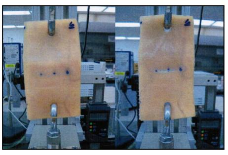
**Figure 2.** An incision closed by LiquiBand (left) and its opening by being pulled apart on the Mark-10 tensiometer.
