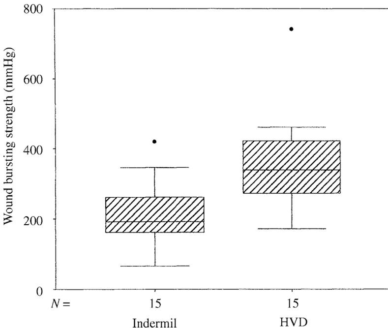
**Figure 1.** Box plots of bursting strength by type of adhesive. The middle bar is the median and the box describes the inter-quartile range. The whiskers approximate the 95% confidence intervals. Outliers are indicated by the individual points. *N* denotes sample size.
